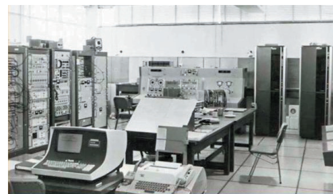
The “tracking” centre. The IRIS control console can be seen in the centre of the picture. The racks on the left monitored the telemetry/data received from the satellite. In the foreground is one of the terminals and next to it is a radio teletype (RTTY) used to receive prediction data. All data received was recorded and sent to France. Source: http://nospremieresannees.fr
