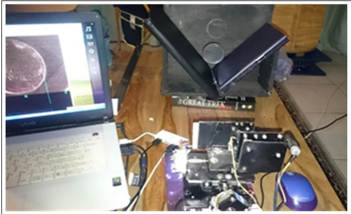
Fig 5. Foucault test setup, with Auto-Foucault tester.
