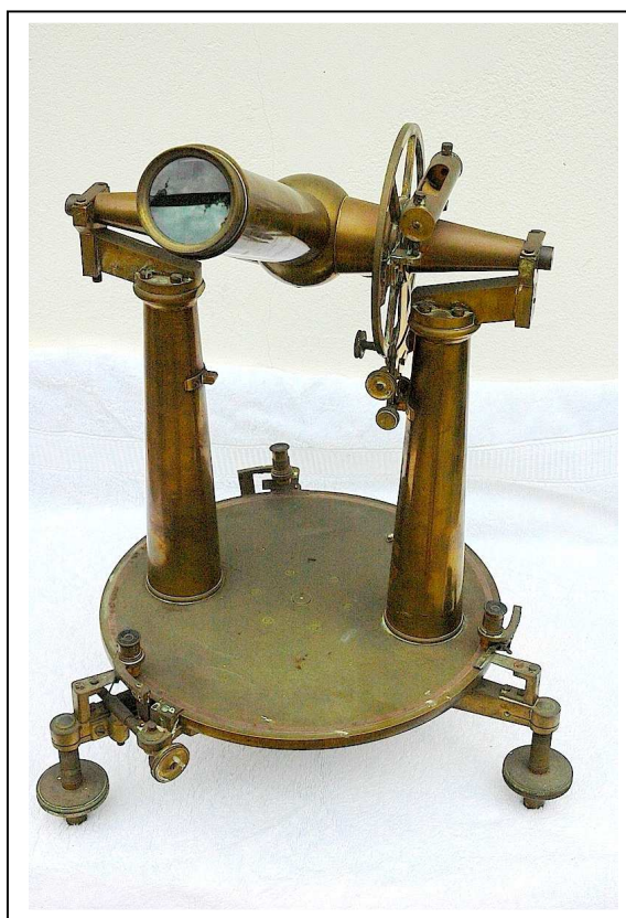
Fig. 4. Troughton & Simms, London, 1839 42 mm solar transit circle. The PEPOS Minutes Book entry dated 16 July 1948 records, "The Royal Observatory, Cape Town is donating a spectroscope, a portable Transit Instrument, and Chronograph, to the People's Observatory. While all are obsolete instruments for research purposes, they are all that is reasonably desired for demonstration purposes."
