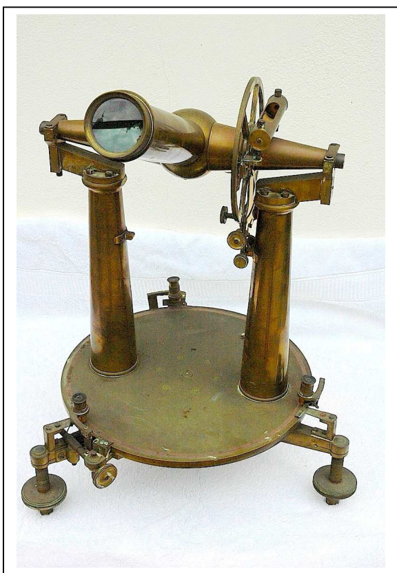
Fig. 4. Troughton & Simms, London, 1839 42 mm solar transit circle. The PEPOS Minutes Book entry dated 16 July 1948 records, "The Royal Observatory, Cape Town is donating a spectroscope, a portable Transit Instrument, and Chronograph, to the People's Observatory. While all are obsolete instruments for research purposes, they are all that is reasonably desired for demonstration purposes."
