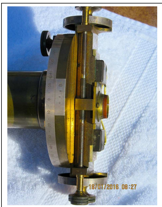
Fig. 2 (left): Cooke 1890s filar micrometer as it came with the Port Elizabeth refractor. In keeping with the elder Cooke's business philosophy that performance delivered must surpass performance claimed, his equipment looked a lot better on a telescope than it did in his catalogue. Photo by the author
