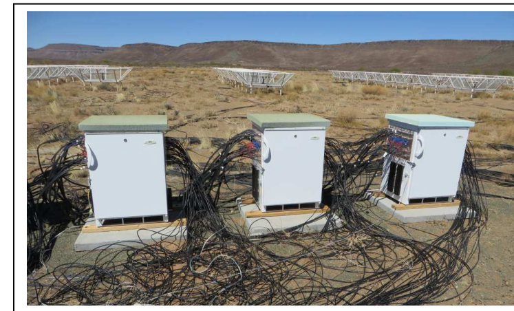
Fig 5. Part of the PAPER array showing where the cables from the 128 telescopes come together.
