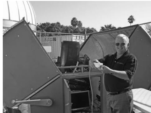
MD Wayne Rosing operating the dome opening paddle of a prototype Aqawan (an Indian word meaning 'to be dry') clamshell enclosure. The production Aqawans will be somewhat larger than this one to house two 0.4m telescopes each. (Picture: Phil Charles)
