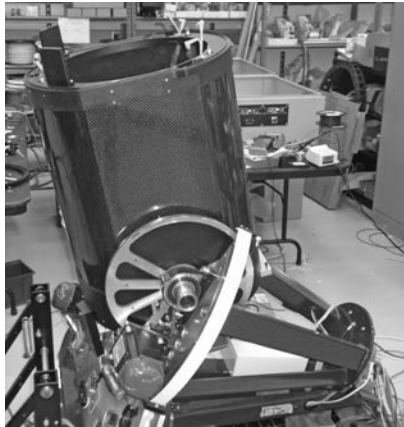
The smaller 16-inch (0.4m) telescopes use the standard Meade telescope tube and optics but is completely customised by LCOGT and mounted on their equatorial split-ring mount. (Pictures: Phil Charles)
