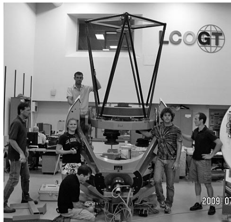
Part of the development team posing with a prototype 1.0m telescope of which 15 will be deployed in the LCOGT network. (Source: LCOGT)
