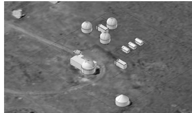
The planned site layout in Sutherland. In the foreground are two existing buildings (a storage rondawel and the IRSF dome) behind which the site will be laid out. Although three buildings of each type are shown here, only two domes and two aqawan enclosures will initially be erected. In 2013 the three best sites in the network will each get an additional 1.0m telescope. The two shipping containers are a site services building (SSB) and storeroom respectively. (Source: LCOGT)
